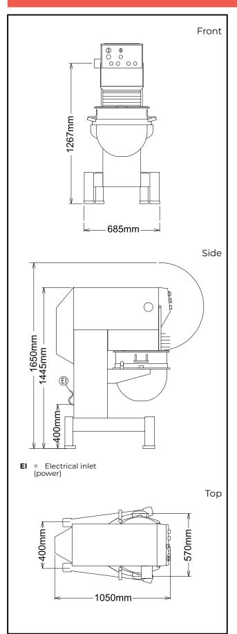
Electric 380-440 V/3N ph/50/60 Hz Supply voltage: Electrical power max: 4 kW **Total Watts:** 4 kW Capacity: ISO 9001; ISO 14001 kg/ Performance (up to): Cycle Capacity: 60 litres Key Information: External dimensions, 685 mm Width: External dimensions, 1050 mm Depth: External dimensions, Height: 1445 mm **Shipping weight:** 324 kg ISO 9001; ISO 14001 kg with Spiral hook **Cold water paste:**
